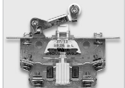
S826 a L / S926 a L Roller lever, mounting brackets, silver contacts, M3 screws with saddle clamp, and magnetic blowout
